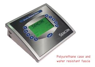
Sencon's Semi-auto Enamel Rater checks lacquer integrity on cans and ends using the industry standard conductivity test. A small, safe voltage is applied between an electrolyte (conductive fluid) inside the can and the body of the can. The amount of resultant current flow indicates the amount of metal exposure caused by any imperfections in the lacquer.
